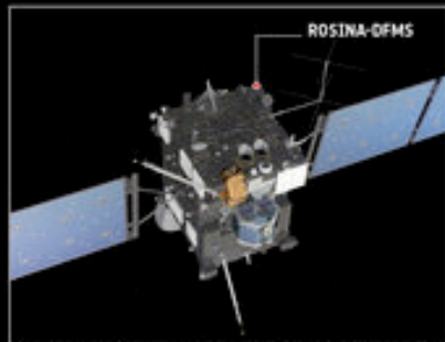
The measurements were made with the Rosetta Orbiter Spectrometer for Ion and Neutral Analysis Double Focusing Mass Spectrometer (ROSINA-DFMS).
